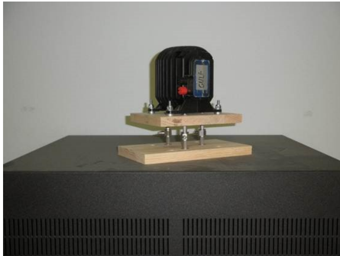
Figure 2.2. Final tactile transducer setup (Photo by K. Grimmelsman)
