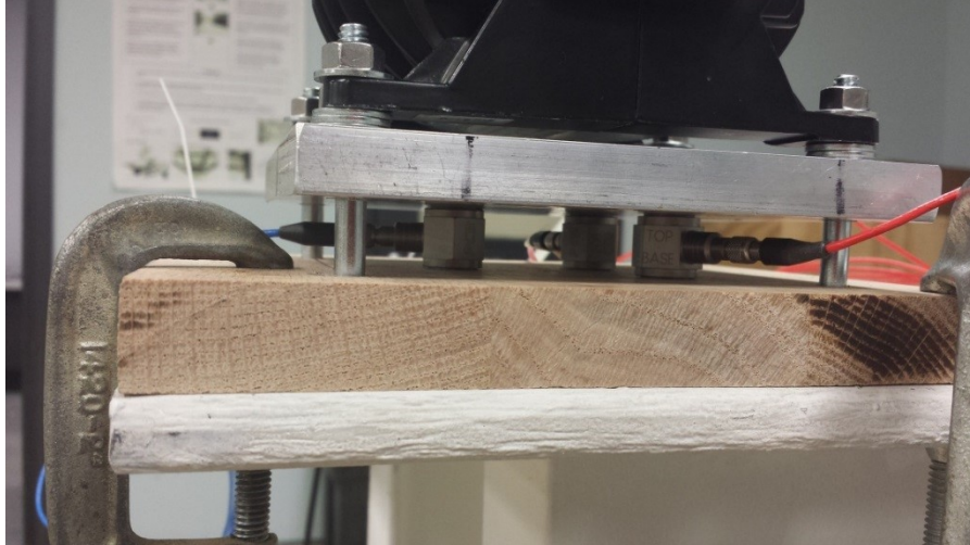
Figure 2.1. Force transducers between stainless steel and wooden plates (Photo by author)
